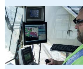
>> Dredging instrumentation Each DOP submersible dredge pump can be fitted out with monitoring equipment. This equipment can be pump-related monitoring such as revolutions, depth and pressure indication. Moreover, the dredging process can be monitored using flow and density meters, vacuum measurement etc.
