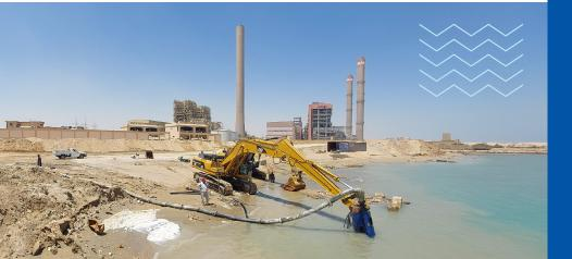
A highly efficient, wear-resistant dredge pump with a large spherical passage is at the heart of the DOP pump. It has excellent suction properties and reaches extremely high mixture densities. The DOP pump has been designed for highly abrasive dredging environments.
