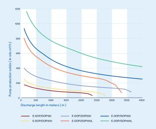
Fine sand,  $D_{so}$ : 0.11 mm, in situ density: 1,900 kg/m<sup>3</sup> At 10m dredging depth and max. 30% concentration. Calculations based on free-flowing sand and no restriction on suction side. Discharge pipe is straight and horizontal with an elevation of 2 meters.
