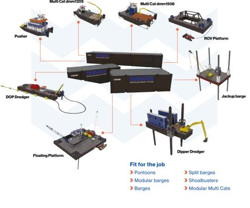
Any dredging job requires support vessels, whether it is a pontoon for easily moving around an excavator with a DOP pump, a number of hopper barges for transporting the dredged sediment, or a customised locally assembled modular vessel or platform using container-sized barge modules. All standard pontoons and barges have a wide scope of usage. The standerdised vessels are available in a range of sizes for use in all waters.
