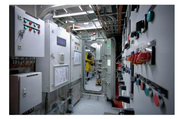
This tank room/control room is seperated from the engine room by means of watertight door.
