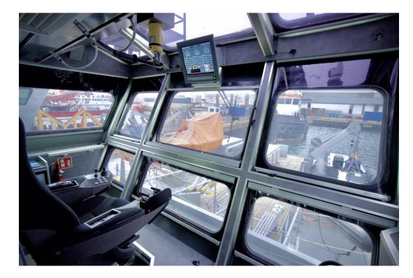
The captain can operate the vessel also from this aft position.
