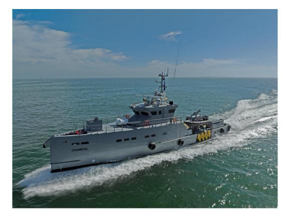
Damen FCS 3307 Patrol Boat Built in 2016 at Damen Shipyards Singapore Dimensions 33.32 x 7.35 x 3.30 m Maximum draft is 2.50 m Aluminium both hull and superstructure Gross tonnage 168
