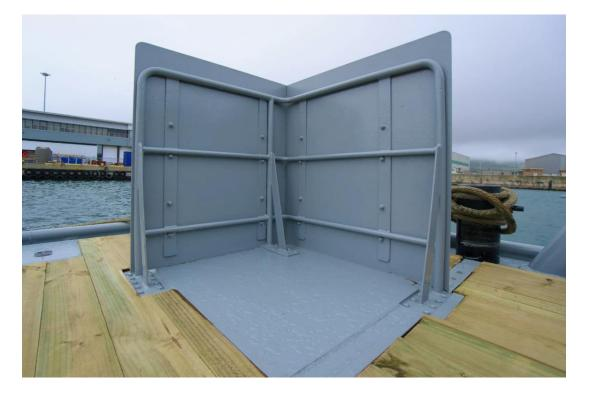
Situated on the aft deck on both PS and SB, armoured protection by means of steel plating.
