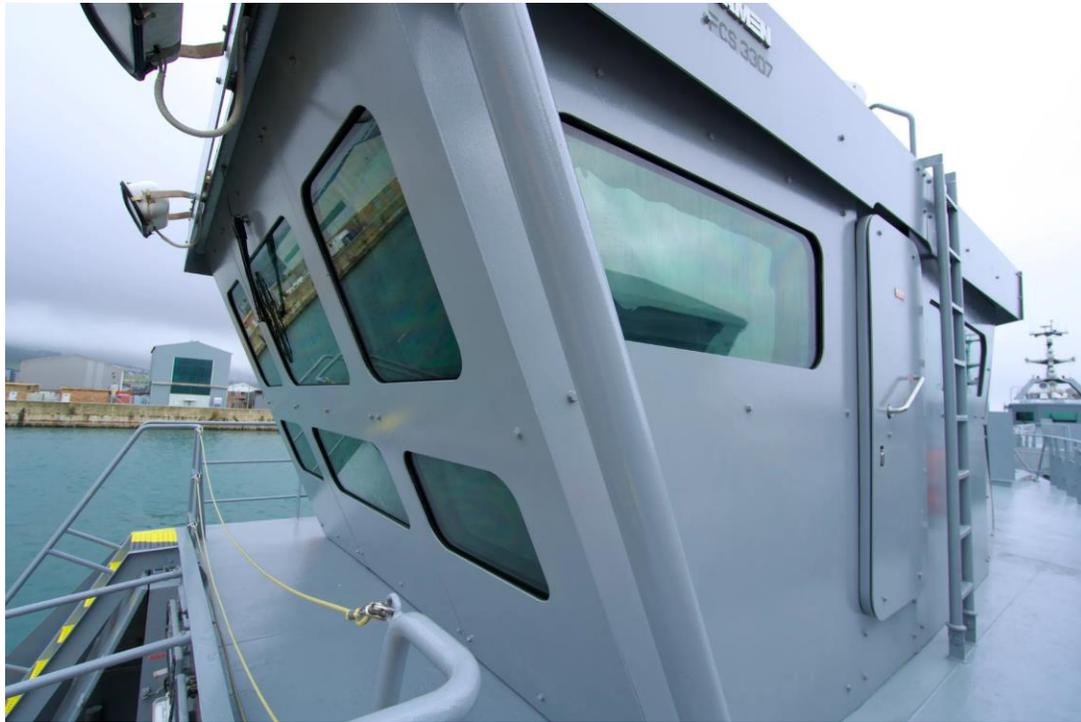
All around the wheelhouse, armoured plating is fitted.
